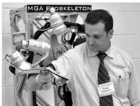
Robotic Rehabilitation —Dr. Carignan places his arm in the exoskeleton system to demonstrate its operation. (Photo by Michael Pearse)
